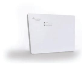
The EN4080 IP gateway combines the functionality of an Inovonics EN4000 receiver with the flexibility of an IP appliance. With a message queuing telemetry transport (MQTT) license, the IP gateway outputs messages in the MQTT protocol. With a BACnet/IP license, the IP gateway outputs messages in the BACnet/IP protocol, which is widely used for building automation and control networks.
