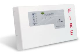
The EH4104R single zone fire RF receiver with relays is designed for use with the Inovonics EH1115EOL EchoStream single input fire RF transmitter to monitor water flow and pressure in piping and post indicator valves to send an alert when a fire protection system has been activated.
